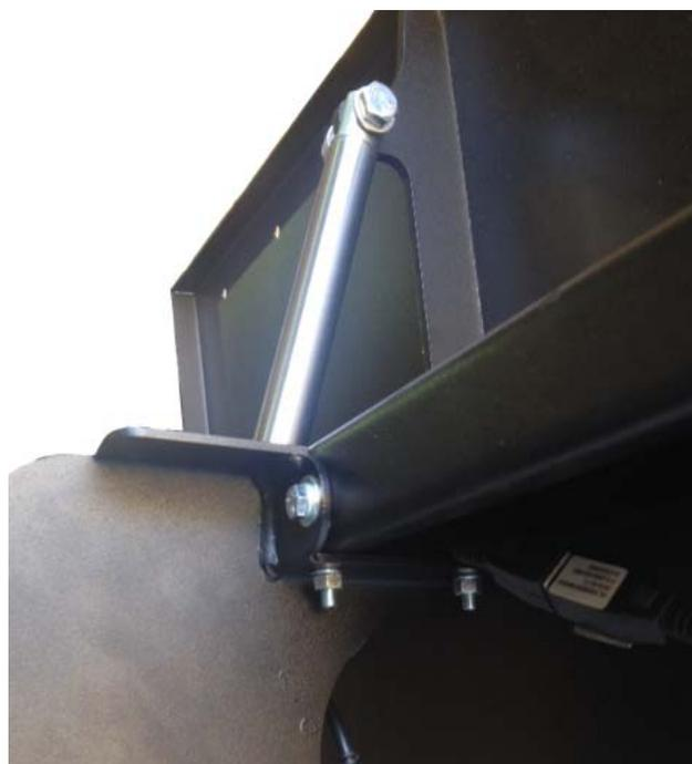
**Step 4:** Now attach the Mounting Plate & Motor to the Base & Supports. Remove the 4 bolts & spring washers from the top of the Hydraulic Supports, position the Mounting Plate & Motor over the Supports, and replace the bolts & washers. NOTE that the Motor Arm must be located on the back side (towards the short base legs) of the Stand. This means the hinge bolts between the Mounting Plate & Mounting Bar are at the front of the Stand, towards the longer base legs.
